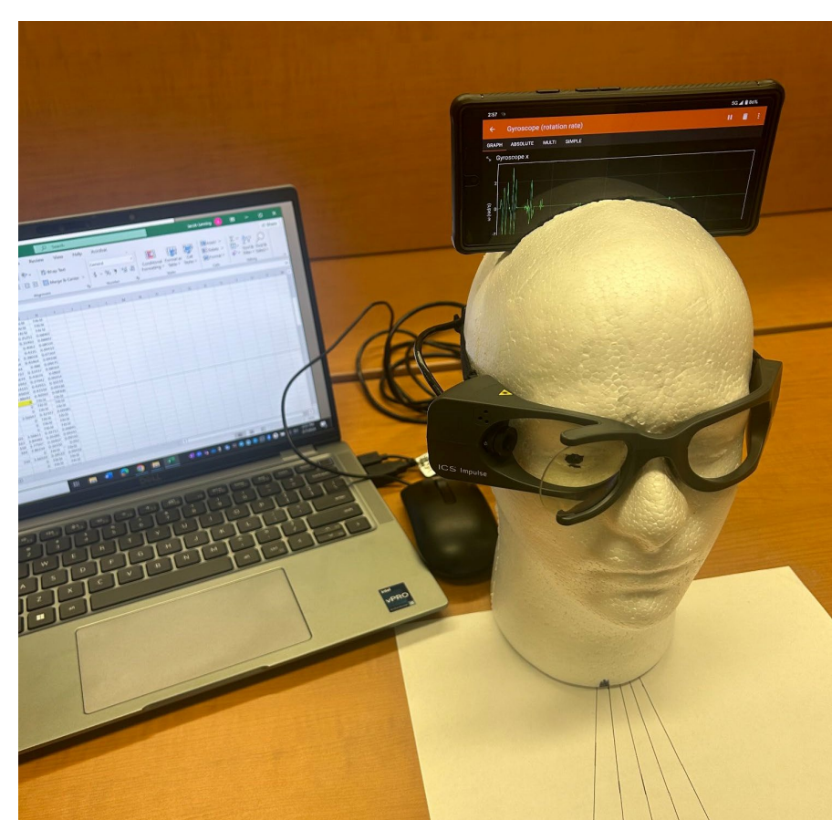
Figure 2: HIT training testing model with smartphone and VOG device in place.
