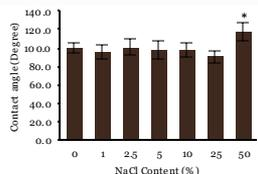
**Figure 2:** The wettability of PEEK discs remained unchanged with increasing NaCl concentrations, except at 50%, where large pores trapped air, increasing hydrophobicity (n=5).
