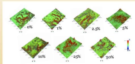
**Figure 4:** Photomicrographs of surface topography of PEEK discs with increased concentrations of NaCl. Red represents high peaks.
