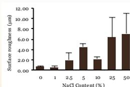
**Figure 3:** The surface roughness of PEEK discs increases with higher NaCl content, peaking at 25% and 50% NaCl, which results in higher surface porosity (n=2).
