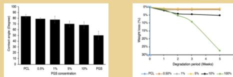
Figure 3: Hydrophilicity Testing and degradation rate of 3D printed scaffolds.
