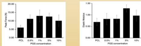
Figure 2: Peak force and elastic modulus of 3D printed scaffolds.
